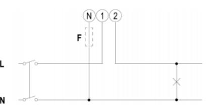
The diagram shows the wiring when used as a grid meter.
